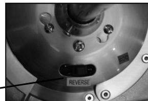
**(15)** The rotor and motor of your fan have been dynamically balanced at the factory. In addition, the blades have been matched to the nearest gram to ensure a well balanced ceiling fan. Furthermore, a blade balancing kit has been included with your fan. Please refer to the instructions packaged with the balancing kit should your fan require additional balancing.
